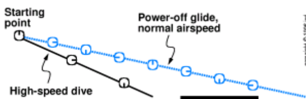
Figure 7.14 : High-Speed Dive versus Normal Glide
