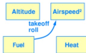
Figure 1.7 : Energy Conversion – Initial Roll
