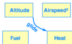
Figure 1.2 : Energy Conversion -- Glide
