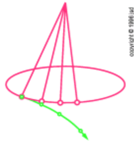
Figure 19.2 : An Object Departing a Centrifuge, with Gravity
