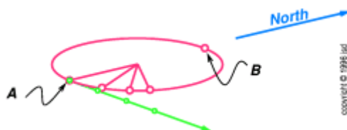
Figure 19.1 : An Object Departing a Centrifuge
