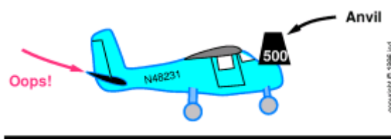
Figure 6.10 : Center of Mass Too Far Forward
