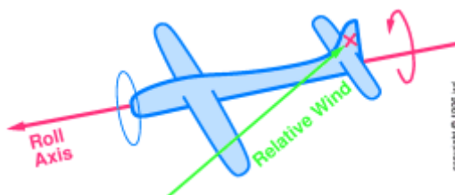
Figure 9.10 : Tall Rudder in a Slip
