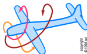
Figure 9.14: Rolling Moment Produced by Propeller
