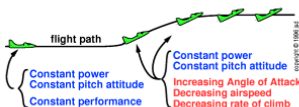
Figure 2.11 : Constant Power & Attitude but Changing Performance
