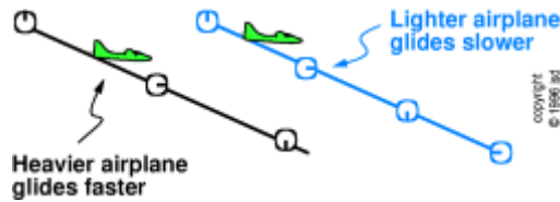
Figure 2.16: Angle of Glide Independent of Weight
