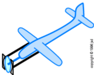
Figure 9.16 : Prony Brake Attached to the Airplane Itself
