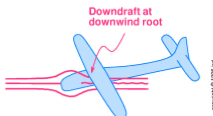
Figure 9.3 : Redirection — High-Wing Airplane in a Slip (1)
