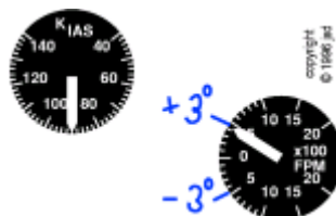
Figure 2.12 : Vertical, Horizontal Speed Gauges Determine Angle
