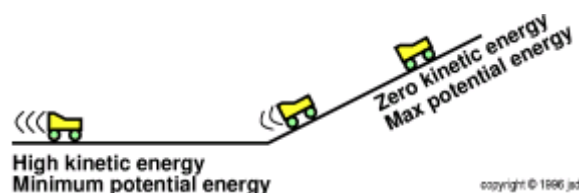
Figure 2.10 : Climb Powered by Speed
