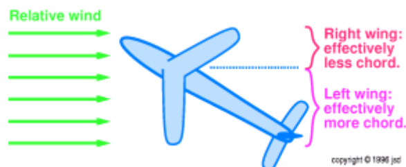
Figure 9.9 : Swept Wing Airplane in a Slip
