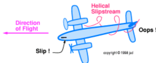
Figure 17.15 : Slip: Helical Propwash Has More Effect
