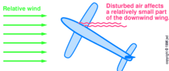
Figure 9.8 : Turbulence — Low-Wing Airplane in a Slip
